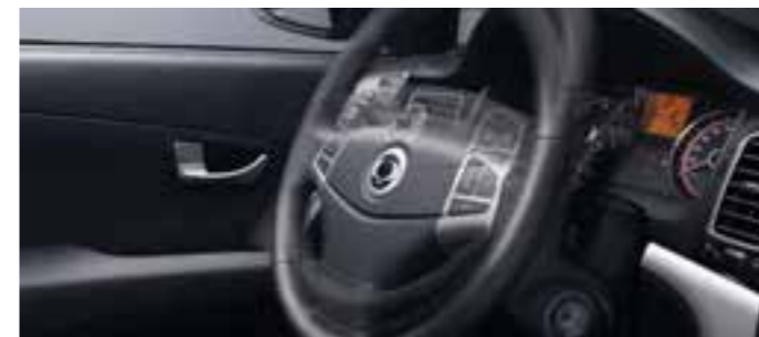
SPEED ADJUSTABLE ELECTRIC POWER STEERING Steering power is heavily assisted in low speed and lightly assisted in high speed to maximize stability and manoeuvrability
