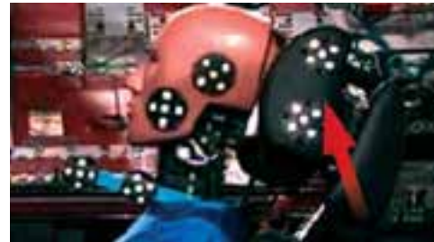
Electronically-activated head restraints Sensors calculate the force of a rear collision and immediately initiate a forward and upward movement of the headrest system to reduce the risk of cervical spine injuries.
