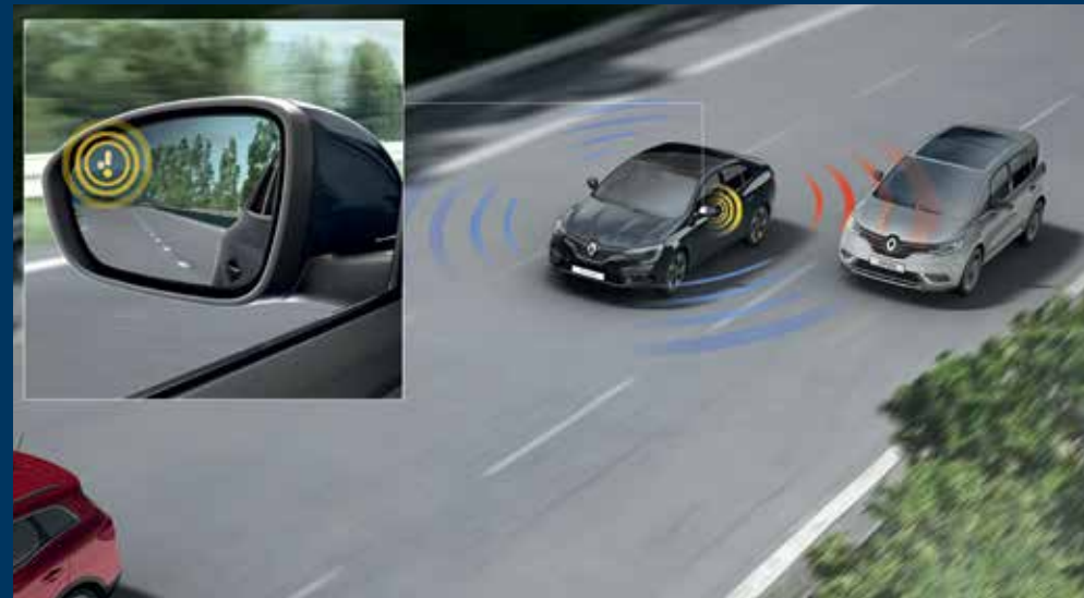
Blind Spot Warning & Moving Object Detection. Be warned against potential collisions with other vehicles to the side and/or to the rear during lane changes between 30 and 140 km/h.
