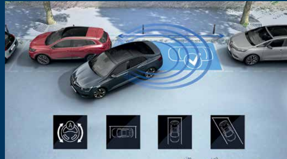
Easy Park Assist. Park with no problem: the system measures the available space and defines the trajectory on its own. Trust it with the steering and admire the manoeuvring.
