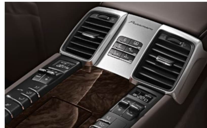
Four-zone automatic climate control
