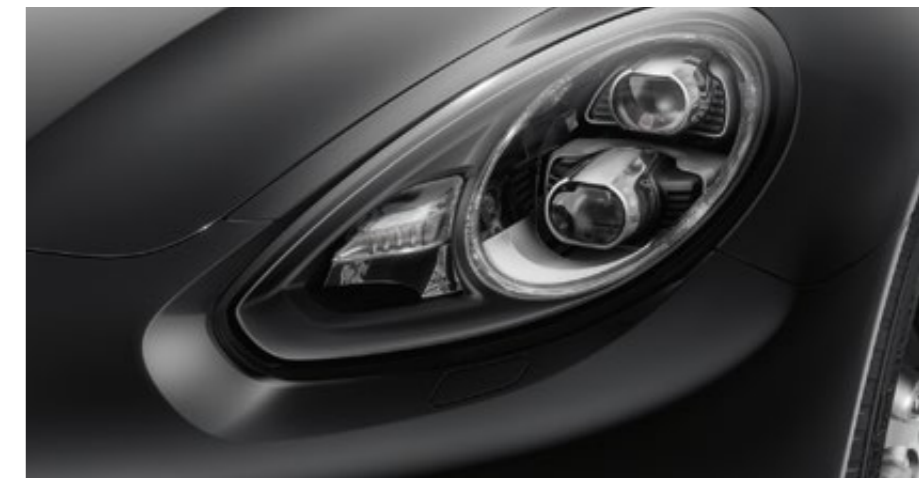
LED main headlight including Porsche Dynamic Light System Plus (PDLS+)
