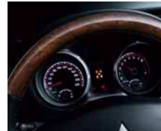
High-contrast back-lit meters and gauges with tachometer, 4WD position display and rheostat 📷 23
