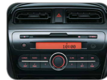
Audio system with clock This unique system includes a digital quartz clock, CD player and AM/FM radio.
