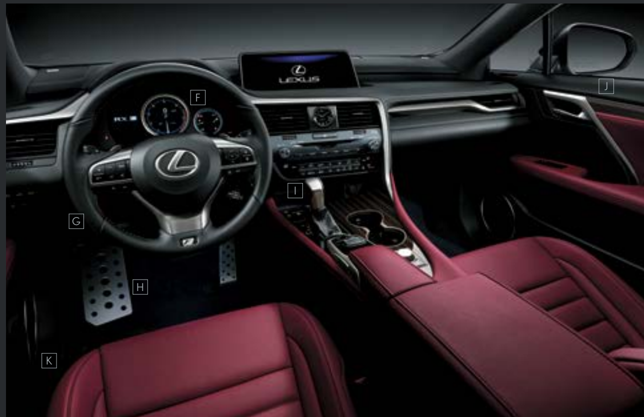
F_Meters & multi-information display / G_Steering wheel / H_Aluminum pedals / I_Shift lever knob / J_Trim (Aluminum) / K_Scuff plates
