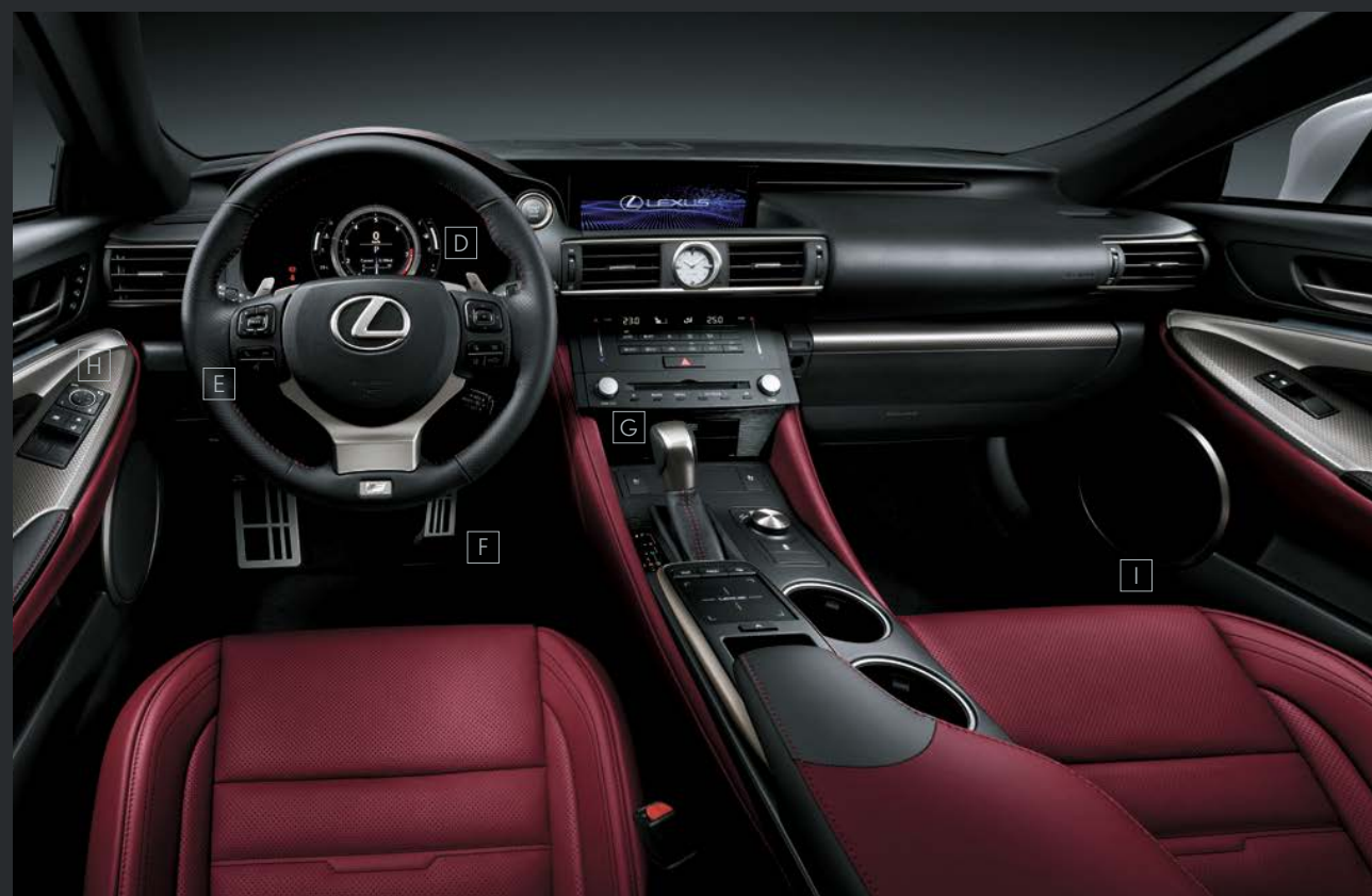
D_Single central meter / E_Steering wheel / F_Aluminum pedals / G_Shift lever knob / H_Trim (Wedge Metal) / I_Scuff plates
