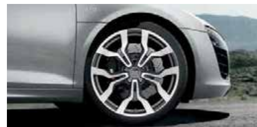
Forged aluminium wheels in 10-spoke Y design, polished, 2-tone size 8.5 J x 19 at front and 11 J x 19 at rear, with 235/35 R 19 tyres at front and 295/30 R 19 tyres at rear
