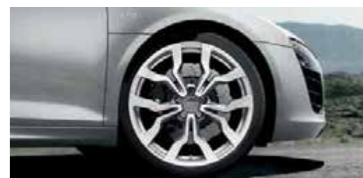
Forged aluminium wheels in 10-spoke Y design, high-gloss polished size 8.5 J x 19 at front and 11 J x 19 at rear, with 235/35 R 19 tyres at front and 305/30 R 19 tyres at rear
