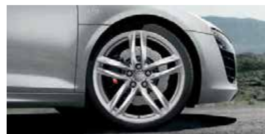
Forged aluminium wheels in 5-twin-spoke design, high-gloss turned finish size 8.5 J x 19 at front and 11 J x 19 at rear, with 235/35 R 19 tyres at front and 295/30 R 19 tyres at rear
