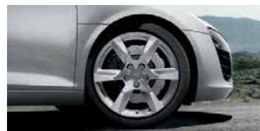
Cast aluminium wheels in 6-arm design size 8.5 J x 18 at front and 10.5 J x 18 at rear, with 235/40 R 18 tyres at front and 285/35 R 18 tyres at rear
