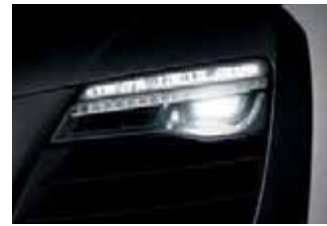
Low beam comprising 6 LEDs plus low beam spotlight
