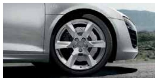
Cast aluminium winter wheels in 6-arm design size 8.5 J x 18 at front, size 10.5 J x 18 at rear, with 235/40 R 18 winter tyres at front and 285/35 R 18 tyres at rear, can be fitted with snow chains, permissible top speed 240 km/h
