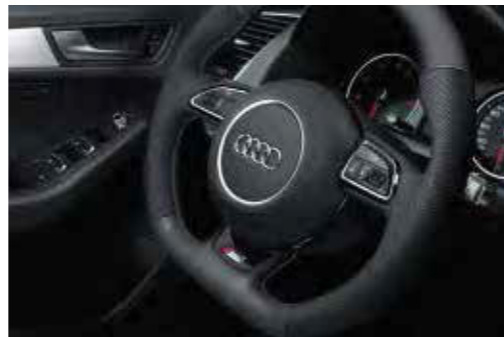
S line leather-covered multifunction sport steering wheel in 3-spoke design, flattened at the bottom
