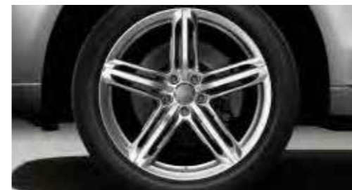
Audi exclusive cast aluminium wheels in 5-segment spoke design size 8.5 J x 20 with 255/45 R 20 tyres, including wheel arch trims. From quattro GmbH
