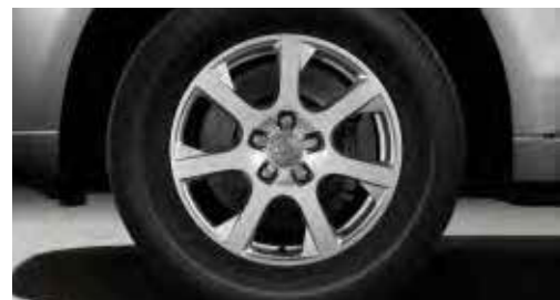
Forged aluminium wheels in 7-spoke design size 8 J x 17 with 235/65 R 17 tyres
