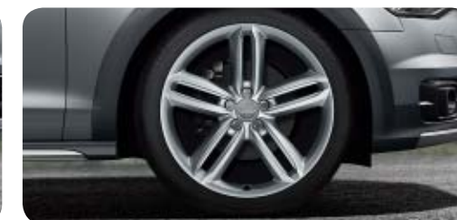
Cast aluminium wheels in 5-parallel-spoke design size 8.5 J x 20 with 255/40 R 20 tyres 1 . Only available for A6 allroad quattro
