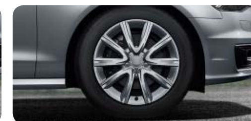
Cast aluminium wheels in 5-V-spoke design size 8 J x 18 with 245/45 R 18 tyres 1
