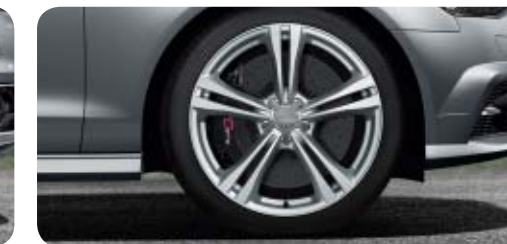
Cast aluminium winter wheels in 5-parallel-spoke star design (S design) size 8.5 J x 20 with 255/35 R 20 tyres 1 , cannot be fitted with snow chains, top-speed suitable. Only available for S6 Saloon and S6 Avant
