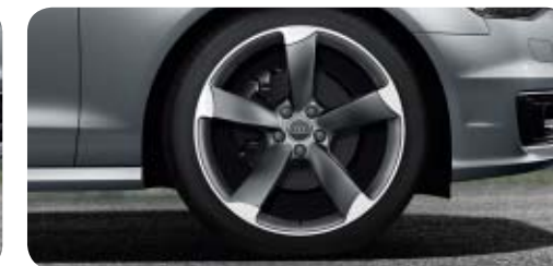
Audi Sport cast aluminium wheels in 5-arm rotor design in matt titanium look, gloss turned finish 2,3 size 8.5 J x 20 with 255/35 R 20 tyres 1
