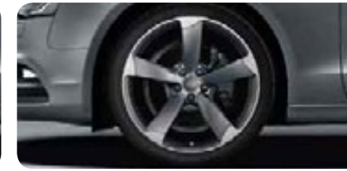
Audi Sport cast aluminium wheels in 5-arm rotor design in matt titanium look, gloss turned finish 2 size 9 J x 19 with 255/35 R 19 tyres 1 . From quattro GmbH
