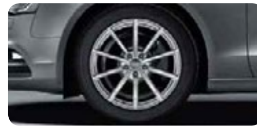
Audi Sport cast aluminium wheels in 10-spoke design size 8.5 J x 18 with 245/40 R 18 tyres 1 . From quattro GmbH
