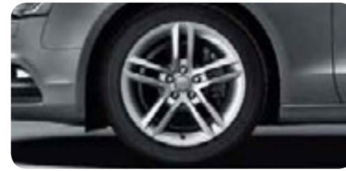
Audi Sport cast aluminium wheels in 5-twin-spoke design size 8.5 J x 18 with 245/40 R 18 tyres 1 . From quattro GmbH
