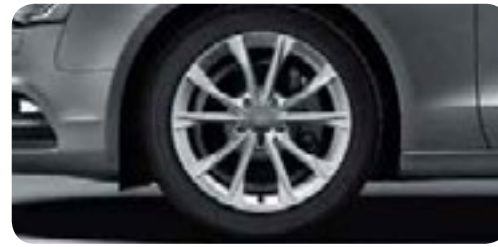
Cast aluminium wheels in 5-V-spoke design size 8.5 x 18 with 245/40 R 18 tyres 1
